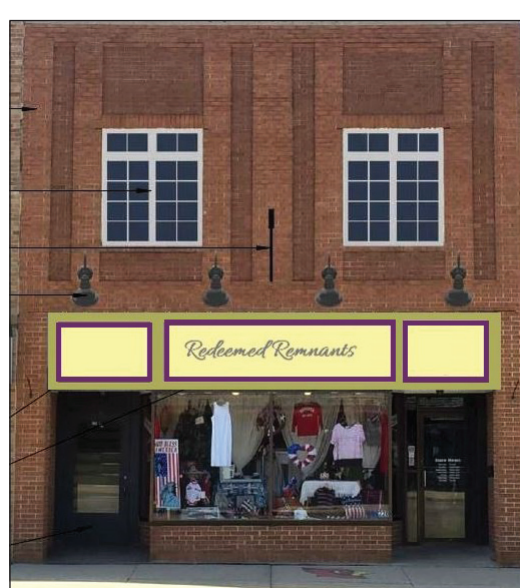
Redeemed Remnants work will include tuck-pointing and cleaning existing brickwork, new windows on the second story, hardy board and composite trim in the sign band area above the storefront windows, new signage and gooseneck lighting and painting and new materials. An architect rendering shows the before and after photos of the proposed project.
