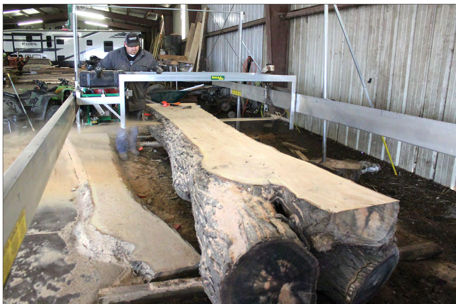
The Lucas Mill used by Ryan Bullerman saws wood logs horizontally of any length but can only safely saw logs 6-feet in height.
