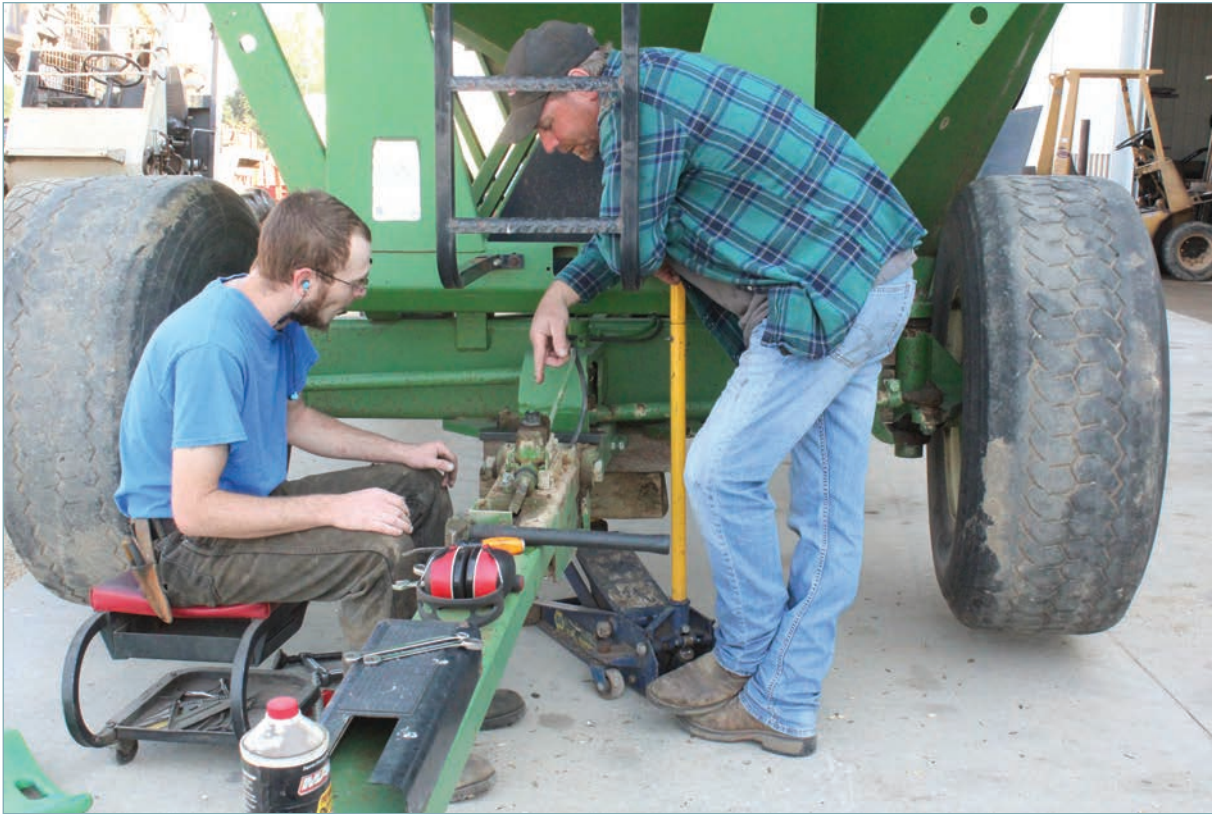
Mert Kracht (right) works with Garritt Beaner to repair a grain truck — setting the brakes, packing the wheel bearings and aligning the wagon. Mert's Repair customers rely on the local welders for all kinds of welding fabrication projects, like this metal tube (at right) Shane Hoag is building for local custom manure haulers to pump manure from livestock pits into tanks. Trevor Kracht cuts a piece of metal for a project.
